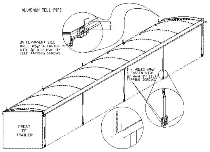
Once the tarp has been secured by the tarp stops, you need to cut off any excess permanent pipe. Cut the permanent pipe 1" past the front and rear of the tarp on the permanent side.
