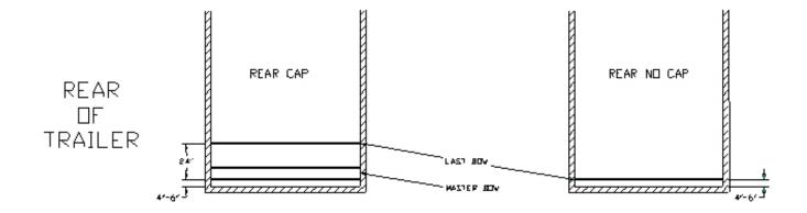
Place the last bow (at the same height) as far back as possible, making sure not to interfere with the operation of the tailgate (must refer to your order form to see what was ordered). If a Rear Cap is used, the last bow will be 24" forward from the <u>back</u> of the Rear Cap. **Make** sure that the installation of the rear bow does not interfere with the opening of the tailgate.
