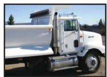
The RCC (Roller, Crank and Canvas) is a manually operated wind up system. It is ideal for light duty trucks, landscaper and stake bodies, and small trailers. The RCC is adjustable in width and can be fitted with a mesh tarpaulin up to 35' long. The system can also be installed with vinyl or drop side tarps. It comes standard with a folding handle and a locking roller.
