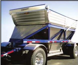
The FLIP'N Go™ Econo is an all aluminum flip system designed for trucks and trailers up to 20' long. The system utilizes the popular spiral spring which has proven to be reliable over the past ten years. The same heavy duty aluminum extrusions that are part of the Flip'N Go™ are used in this system. The FNG Econo is lighter in weight and less expensive. It is available in a manual or electric version.
